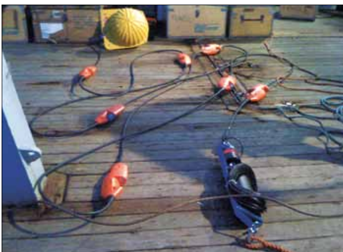
Fig. 3: UGOT Seaguard with 20 m string on-deck before deployment. Measures: Currents at one level, Water level, Cond/Sal/Temp at 4 levels, O 2 /Temp at 3 levels. There is empty space for 11 additional sensors. The autonomy of the system is about 1 year using internal batteries and set to record data at 20 min intervals.
