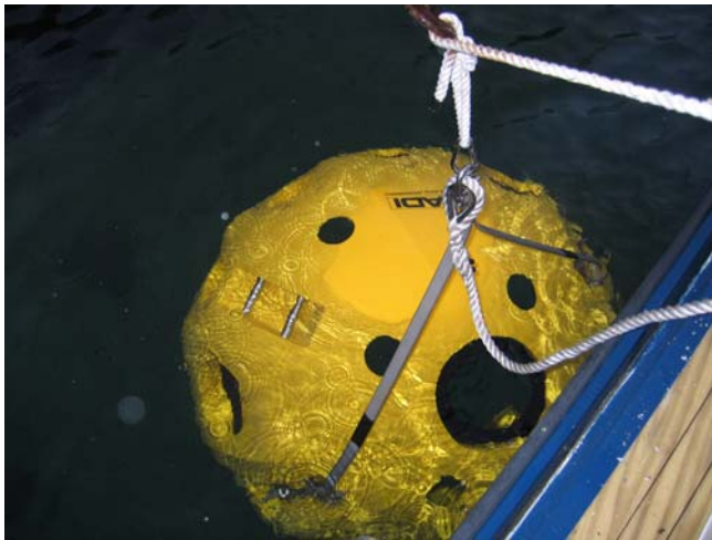
Figure 4-3 Fixed Bottom Mooring Frame 3448. The picture is taken during a test deployment.
