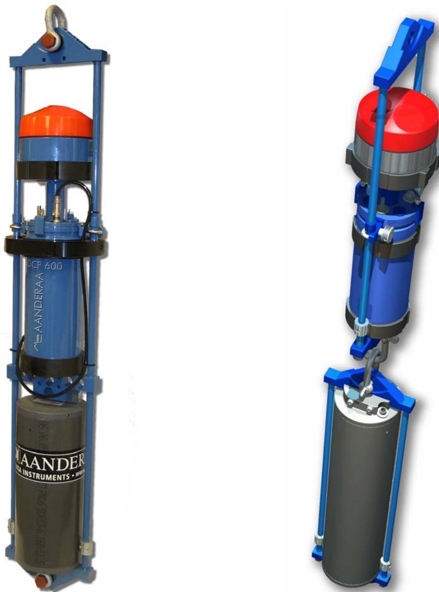
Figure A- 1 left: Extended in-line mooring Frame 4110 with a complete battery case 4062 (300m version) and an RDCP600. Cable 3997S for connection. Right: Drawing of In-line mooring frame with Battery case 5062 and In-line mooring frame 3910A with RDCP600.
