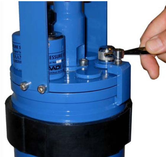
Figure 4-9 Tighten C-clamps until the pressure case rotates on the floor. Avoid over tightening as this will bend the C-clamps.
