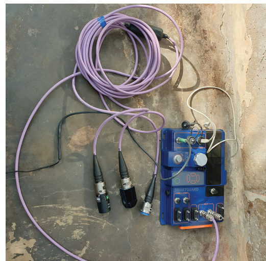
Figure 2: During the selection for suitable dissolved oxygen and temperature sensor, Aanderaa 4835 Optode and 4319 Conductivity sensor connected with Smartguard were deployed and tested in the Vertical Oceans' facility.
