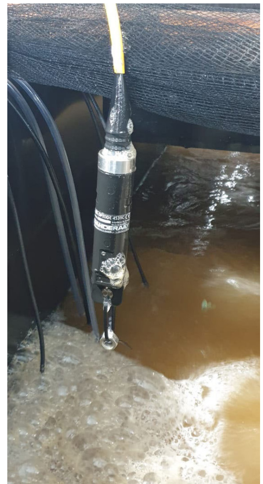
Figure 1: Aanderaa AquaOptode 4531 deployed in shrimp tank for continuous dissolved oxygen and temperature measurements.
