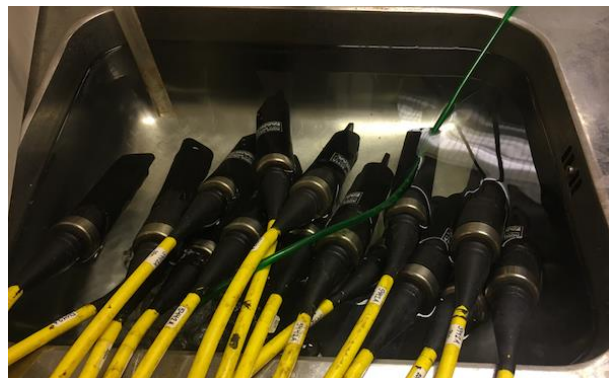
Fig. 1: Sixteen (16) optodes immersed into air-bubbled freshwater for post-deployment calibration check.
