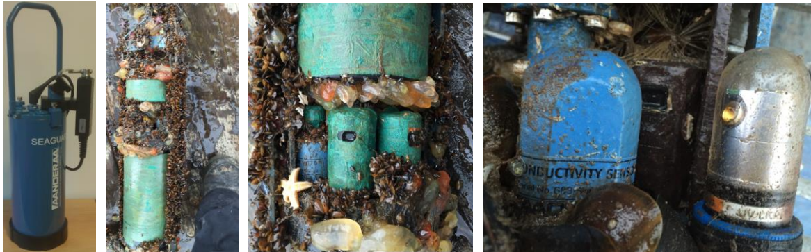
Figure 4, Left: Wiper protecting of a pCO 2 optode against fouling, wiping is activated by one of the four SeaGuard analog ports. Middle left: multi-parameter instrument with copper tape on some parts after 2 months in an area with high biofouling. The copper tape last for about 1 year and nothing grows on it. Middle right: Close-up of the Turbidity and O 2 optode both measured correctly for 1 and 2 months respectively. Right: Conductivity and O 2 optode on SeaGuard were successfully bio fouling protected by UV-LED's during the active season.
