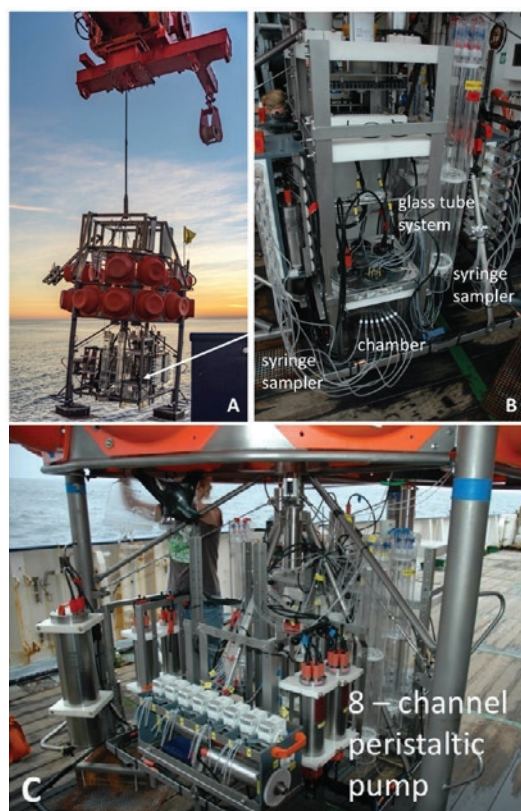
Figure 11 A. GEOMAR BIGO Lander (Biogeochemical Observatory) for benthic flux measurements with Launcher unit mounted on its top, B. detail view of one benthic flux chamber, C. detail view of scientific payload and the 8 channel peristaltic pump for water sampling.
