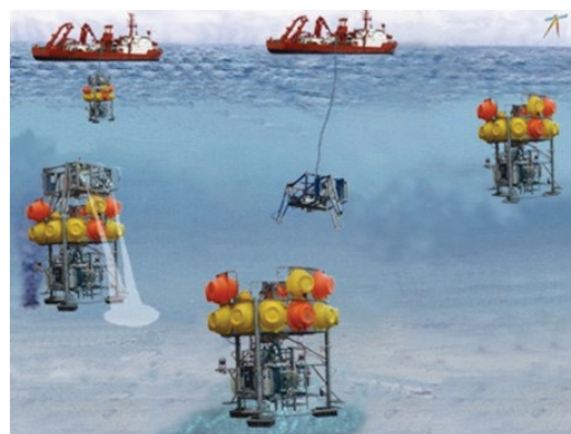
Figure 10: Geomar's real-time video release system makes it possible to place the lander precisely on the seafloor.
