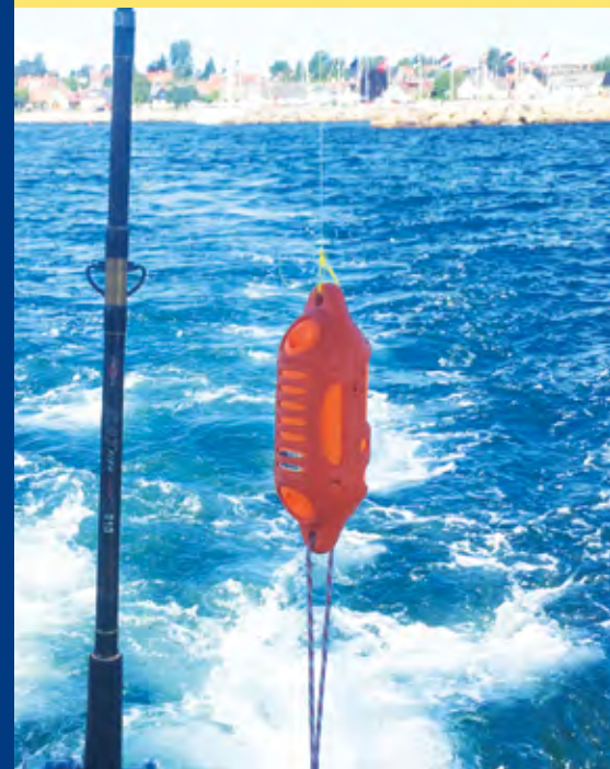
SonTek CastAway CTD deployed via a fishing rod at regular intervals.
