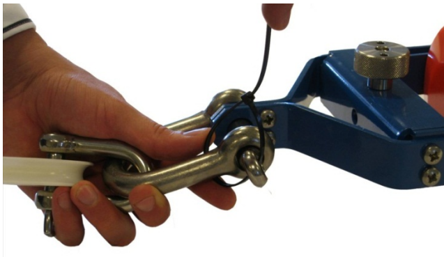
Figure 6-6 Lock the shackle with strips or locking wire. Locking wire is recommended for higher security in long deployments.
