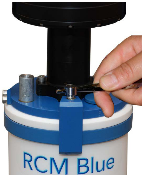
Figure 6-2 Tighten C-clamps until the pressure case rests on the Top-End plate. Avoid over tightening as this will bend the C-clamps.
