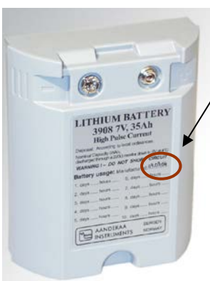
Figure 6-18 Check the manufacture date
