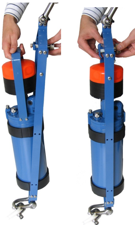
Figure 6-3 Mount the instrument into the frame. Illustrated with a Seaguard RCM.
