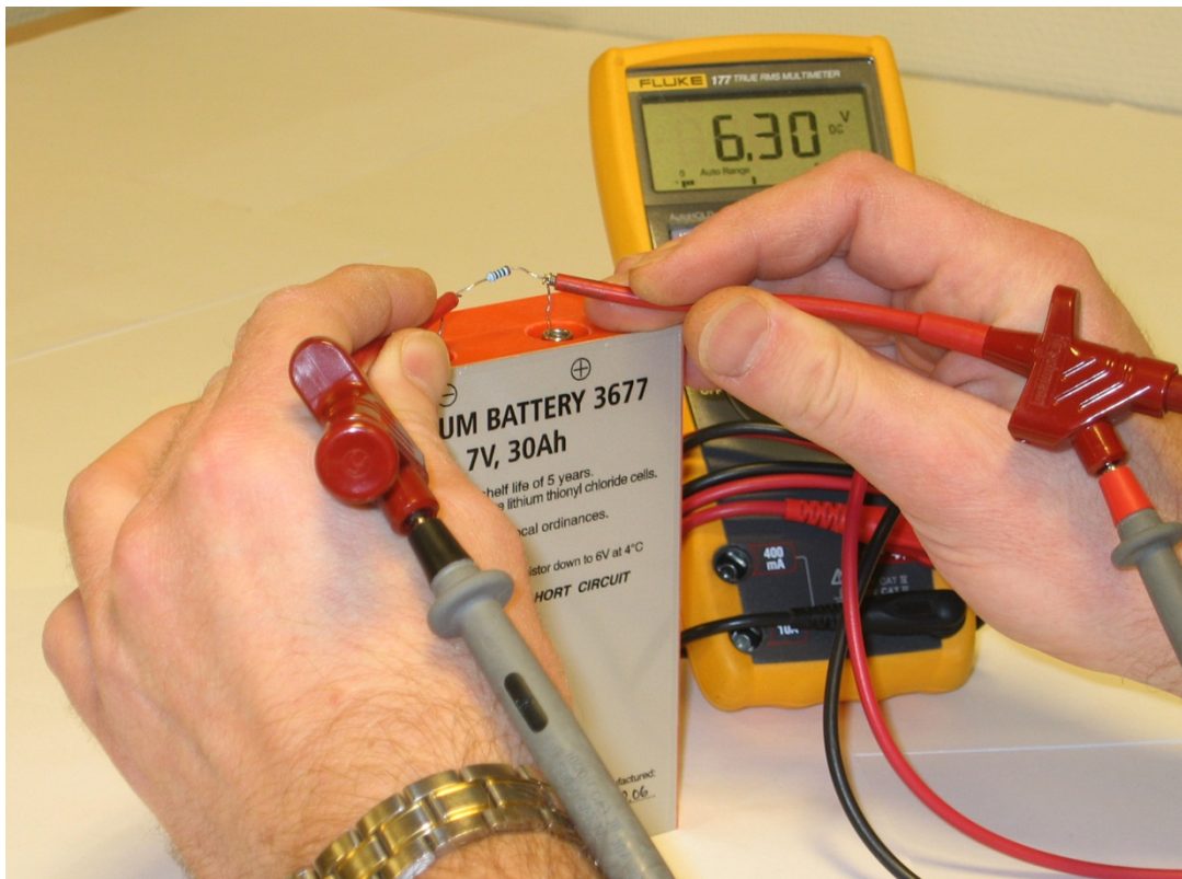
Figure 6-19 Use a 100 \Omega resistor up to 6.3 V to rejuvenate the battery. Note! Illustration shown with older Lithium batteries; today's batteries has connection pins at the side, not on top.
