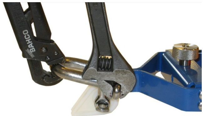
Figure 6-4 Fasten shackle in frame. Tighten thoroughly.
