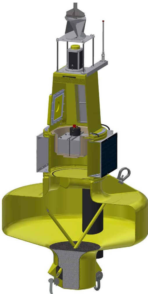
Figure 10-4: Battery and sensor location
