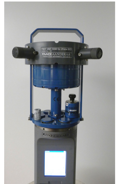
Test Unit connected to SeaGuard with display
