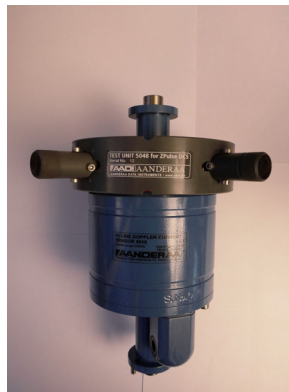
Test Unit connected to In-line DCS
