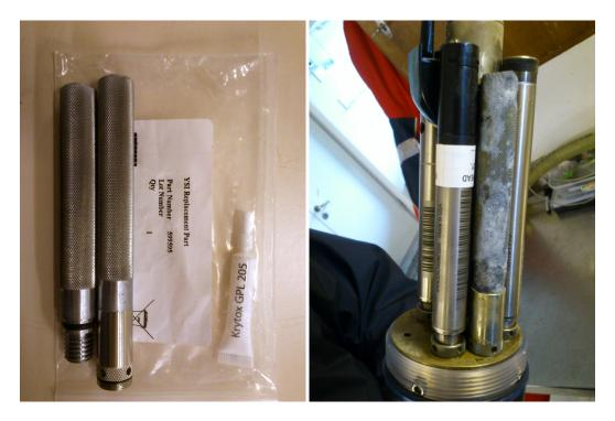
Figure 4: YSI EXO2 sonde, sacrificial anode before and after deployment (6 months under water).
