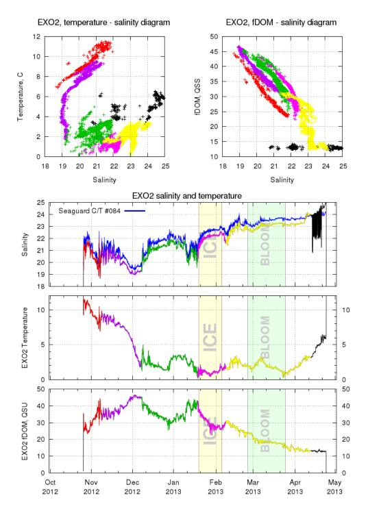
Figure 17: EXO2 temperature, salinity, and fDOM as indicators of water exchange/mixing.
