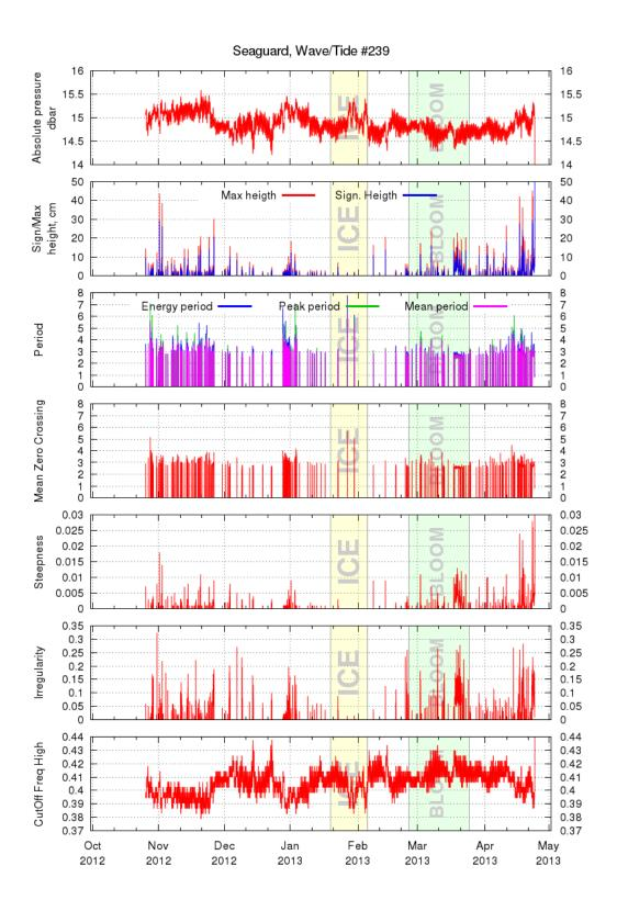
Figure 15: Seaguard Wave/Tide sensor #239 data. A period with strong waves in mid-March 2013 at the end of the bloom.
