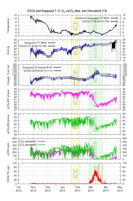
Figure 12: Seaguard and EXO2. T, S, oxygen,  $CO_2$ , TA and BGA Chlorophyll data.  $O_2$  supersaturation peak during the bloom corresponds to the minimum on  $CO_2$  data. Raw  $CO_2$  data look good, but calibration for  $CO_2$ optode #21 is most likely not valid.
