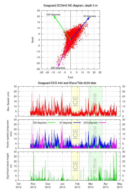
Figure 16: Seaguard DCS #43 and Wave/Tide #239, current and wave data. Very weak currents under ice. A period with strong waves in mid-March 2013 at the end of the bloom.
