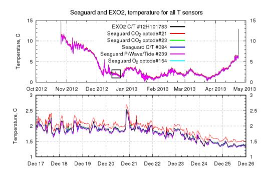
Figure 7: EXO2 and Seaguard, temperature from all sensors.  $pCO_2$  optode #21 readings were always higher by 0.15 C. All other T sensor readings seem to agree very well.
