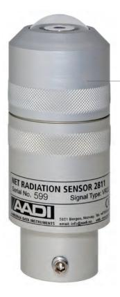
Net radiation is an important parameter in meteorological, climatological and agricultural studies. The 2811 sensor measures both sunlight and infrared radiation, and it is a standard sensor for the Aanderaa Automatic Weather Station 2700. It is rugged, stable and will operate under all weather conditions.
