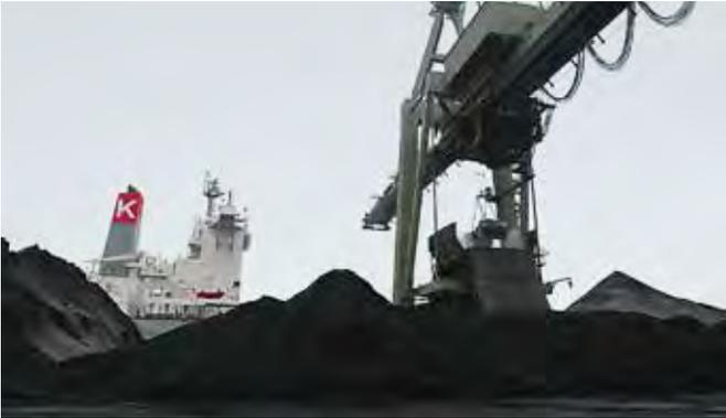
The quay system at EMO is equipped to receive the world's largest bulk carriers. Here a ship is unloaded using two cranes. The daily unloading capacity at the terminal is 200,000 tonnes.
