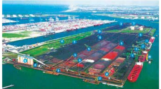
EMO is Europe's largest terminal for coal and iron ore. The enterprise occupies 160 hectares and has a capacity for 60 million tonnes annually. Last year 35 million tonnes passed through the plant.
