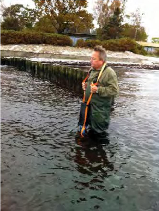
*Mapping of O<sub>2</sub>/Temp/Sal in and around the algae belt by walking.*
