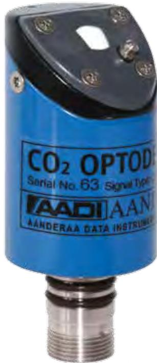
The new CO<sub>2</sub> Optode uses fluorescent dual lifetime detection of pH. When CO<sub>2</sub> diffuses into a gas permeable foil the pH in an embedded buffer will change, subsequently changing the fluorescence of the pH sensitive indicator.
