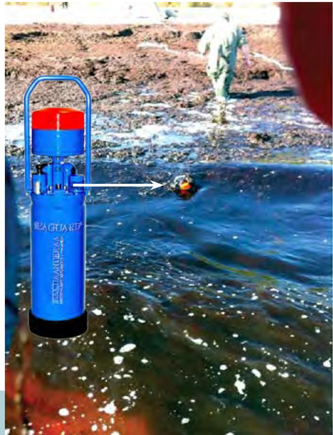
*Pushing the SEAGUARD® into the sediment at the rim of the bet leaving the sensors 10-15 cm above the sediment surface.*
