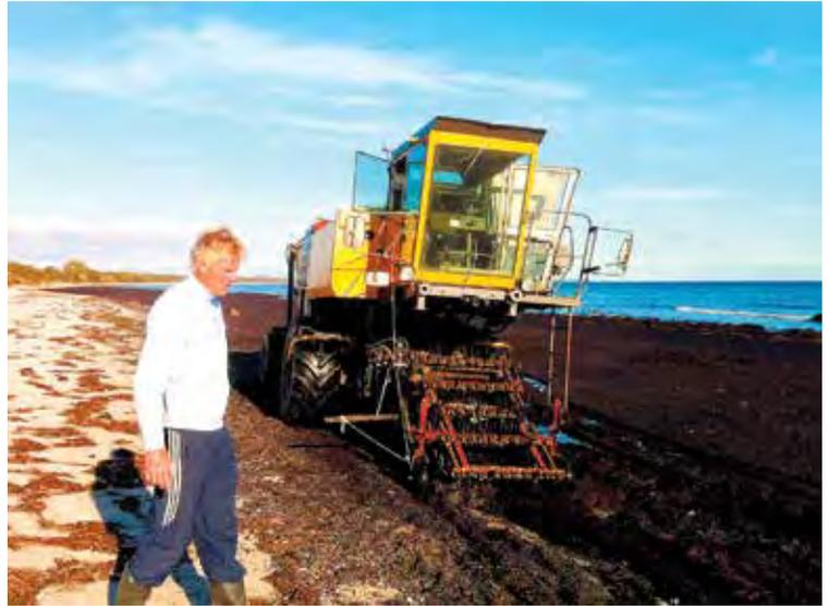
Fig 1: A rebuilt pea harvesting machine is used to gently collect algae excluding as much beach sand from the biomass as possible.
