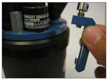
Carefully lift the instrument main module out of the pressure case.
