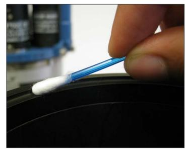
Remove old o-ring. Do not use sharp tools (it may damage the o-ring groove and cause water intrusion)!
