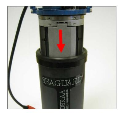
Rotate the instrument main module ½ turn in the pressure case.
