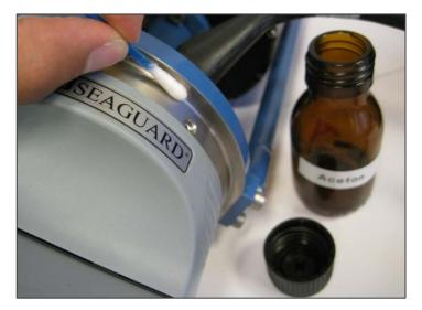
Inspect o-ring grooves. Preferably use a bright lamp and a magnification device. Check for unremoved particles and scratches.
