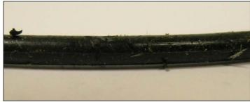
Apply new grease to o-ring.
