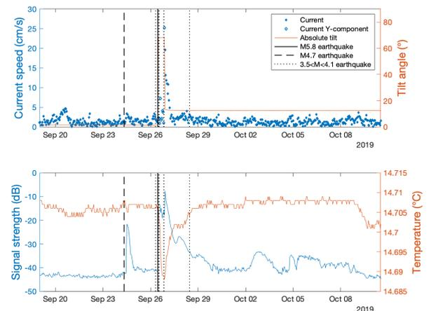
Figure 2. Time series acquired with a Doppler Current Sensor (DCS) on a SeaGuard during the September 2019 seismicity cluster; (top) current speed and tilt; (bottom) backscatter signal strength and temperature (figure from Henry et al 2022).
