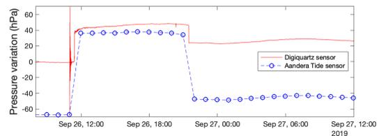
Figure 3: Pressure variations recorded by two instruments around the time of occurrence of a Mw 5.8 earthquake (figure from Henry et al 2022).
