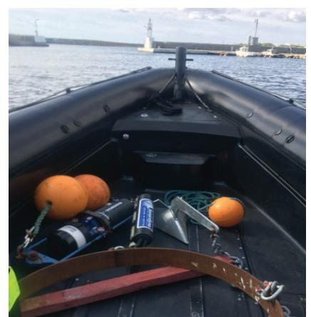
Figure 3: SeaGuardII mooring on its way to the deployment site. Deployment and recovery is done manually and takes less than 10 min each.
