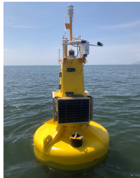
A MOTUS buoy equipped with solar panels and sensors floats on Lake Victoria—delivering real-time data for safer navigation and environmental monitoring.
