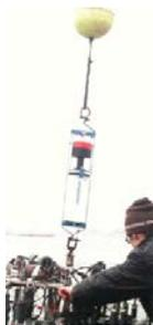
**RCM Blue:** First presented last year [RCM Blue](#) has quickly gained its position as a price effective alternative for a top quality coastal current meter. It is self-recording equipped with Bluetooth for set-up and data retrieval without opening. It measures currents with Z-pulse technology and temperature. It features exceptional battery capacity compared to other alternatives.
