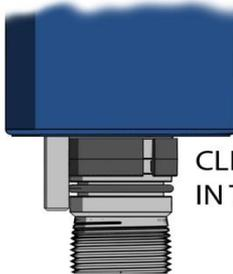
CLIP ON PLASTIC RING IN TOP O-RING GROOVE
