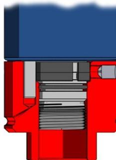
PUT ON ADAPTER AND TIGHTEN SET SCREW
