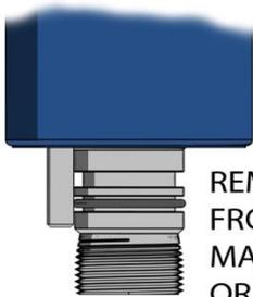
REMOVE TOP O-RING FROM THE SENSOR FOOT MAKE SURE THE ORIENTATION PIN IS IN PLACE
