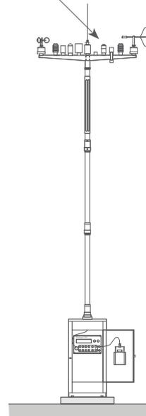
Net radiation is an important parameter in meteorological, climatological and agricultural studies. The 2811 sensor measures both sunlight and infrared radiation, and it is a standard sensor for the Aanderaa Automatic Weather Station 2700. It is rugged, stable and will operate under all weather conditions.
