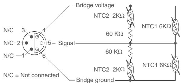
NTC1: Thermistor Unicurve 6 k $\Omega$  at 20°C
