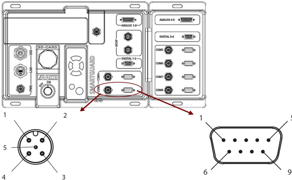
Figure A 4 4-pin M12 and 9-pin D sub connection plug. Refer Table A 5 and Table A 6 for signal wiring.
