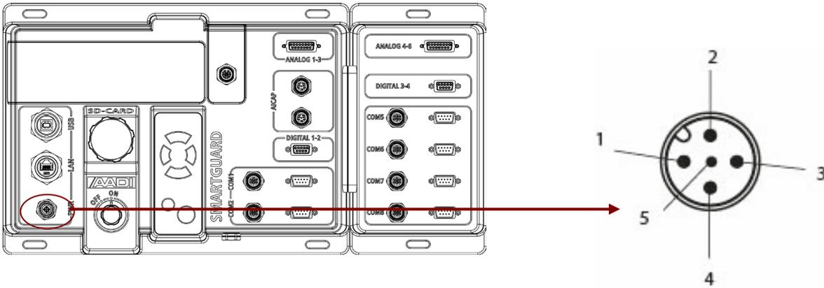
Figure A 2 4-pin M12 power plug. Refer Table A 2 for signal wiring.
