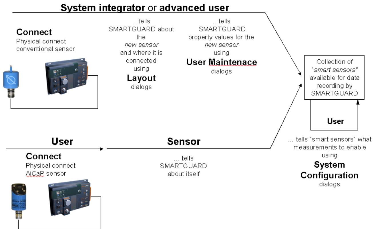
Figure 2-1 Sensor integration with SmartGuard.
