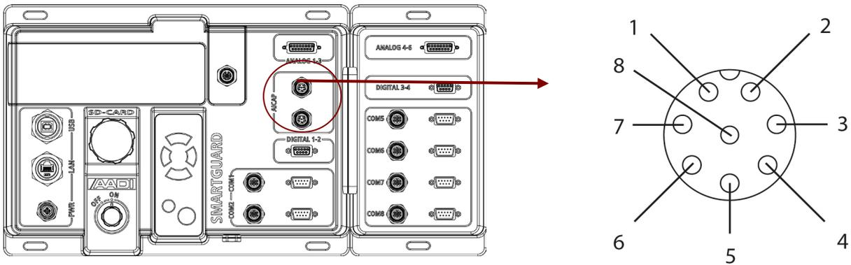
Figure A 7 8-pin M12 connection plug. Refer Table A 9 for signal wiring.
