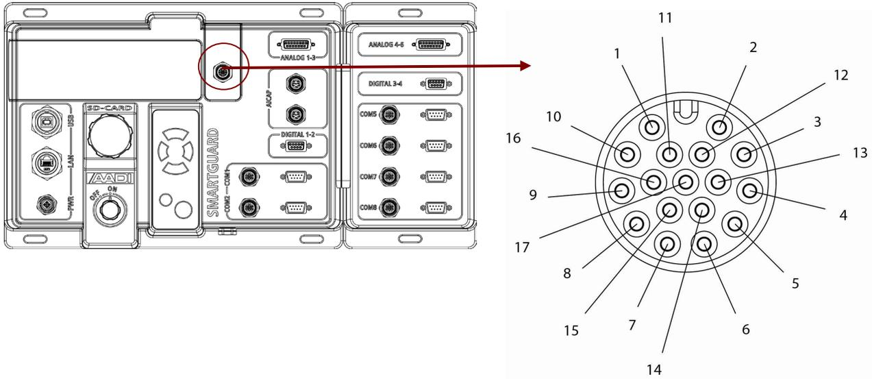
Figure A 8 17-pin M12 connection plug. Refer Table A 10 for signal wiring.
