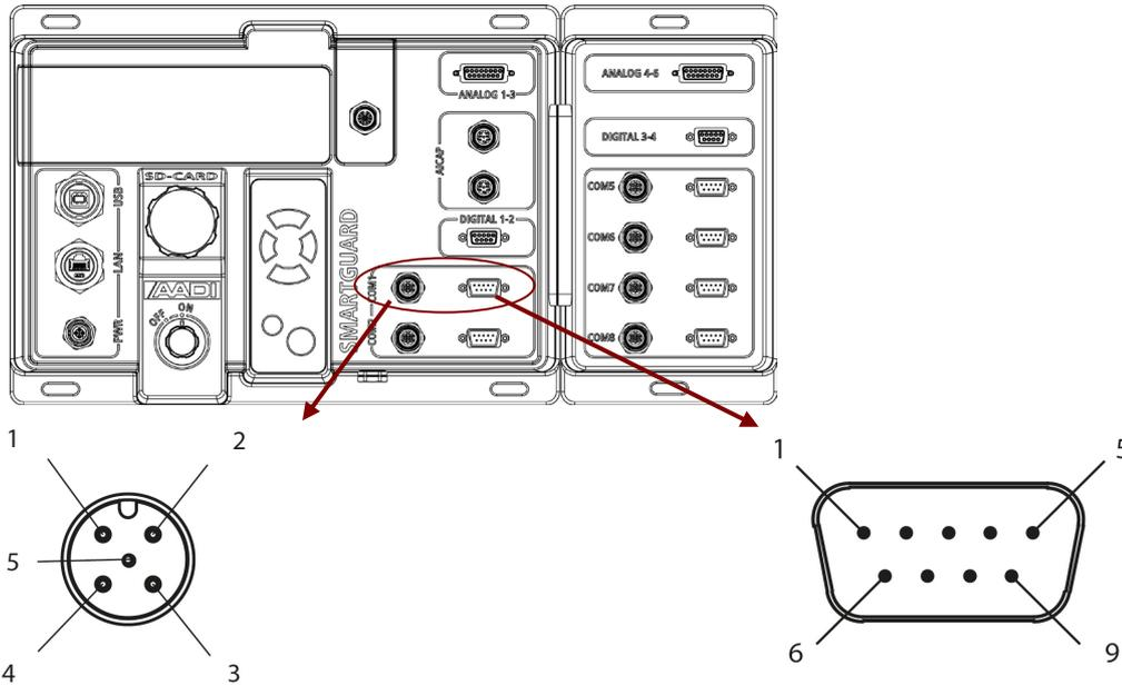
Figure A 3 4-pin M12 and 9-pin D sub connection plug. Refer Table A 2 - Table A 4 for signal wiring.
