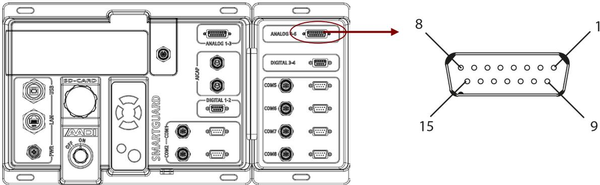
Figure A 13 9-pin D sub connection plug. Refer Table A 18 for signal wiring.
