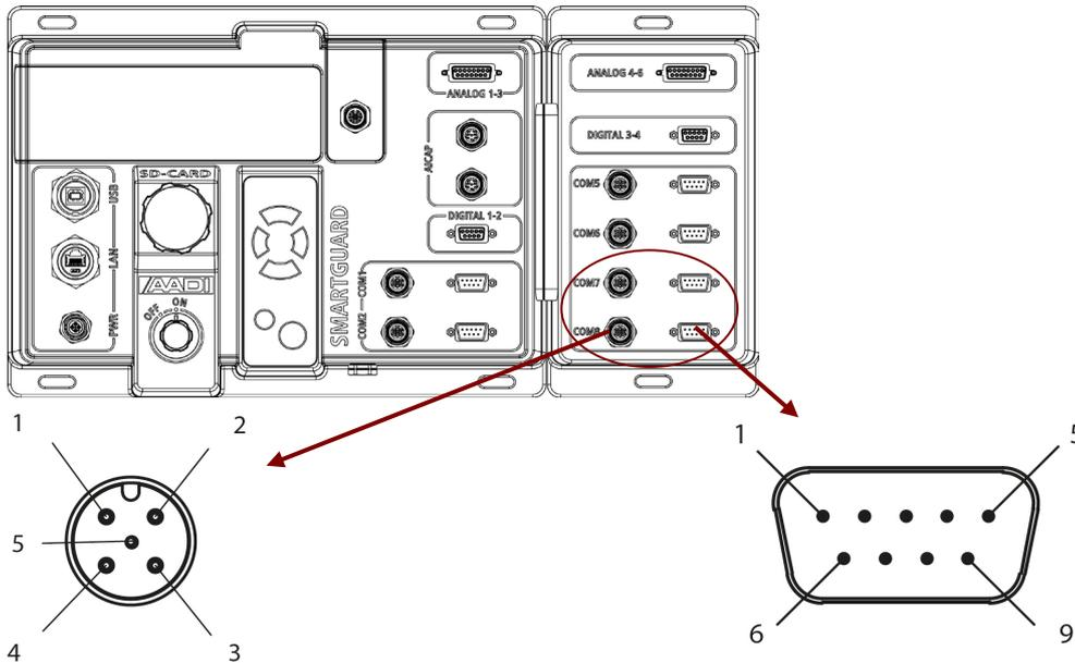
Figure A 11 4-pin M12 and 9-pin D sub connection plug. Refer Table A 14 - Table A 16 for signal wiring.
