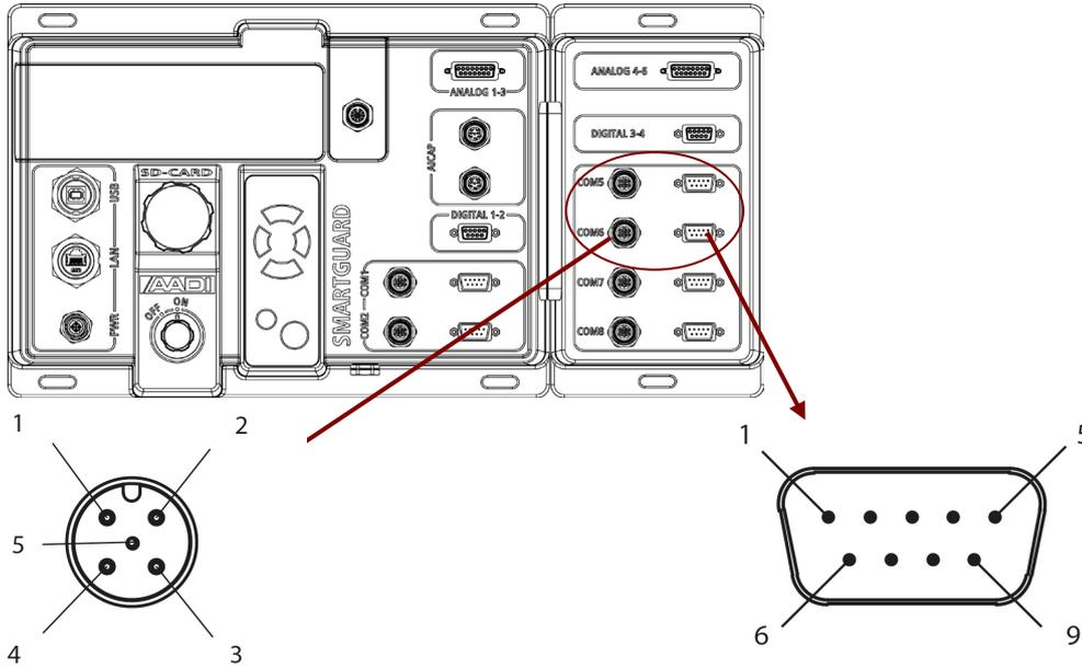
Figure A 10 4-pin M12 and 9-pin D sub connection plug. Refer Table A 12 and Table A 13 for signal wiring.
