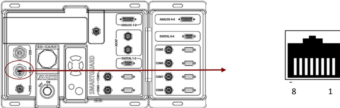
Figure A 9 RJ45 connection plug. Refer Table A 11 for signal wiring.
