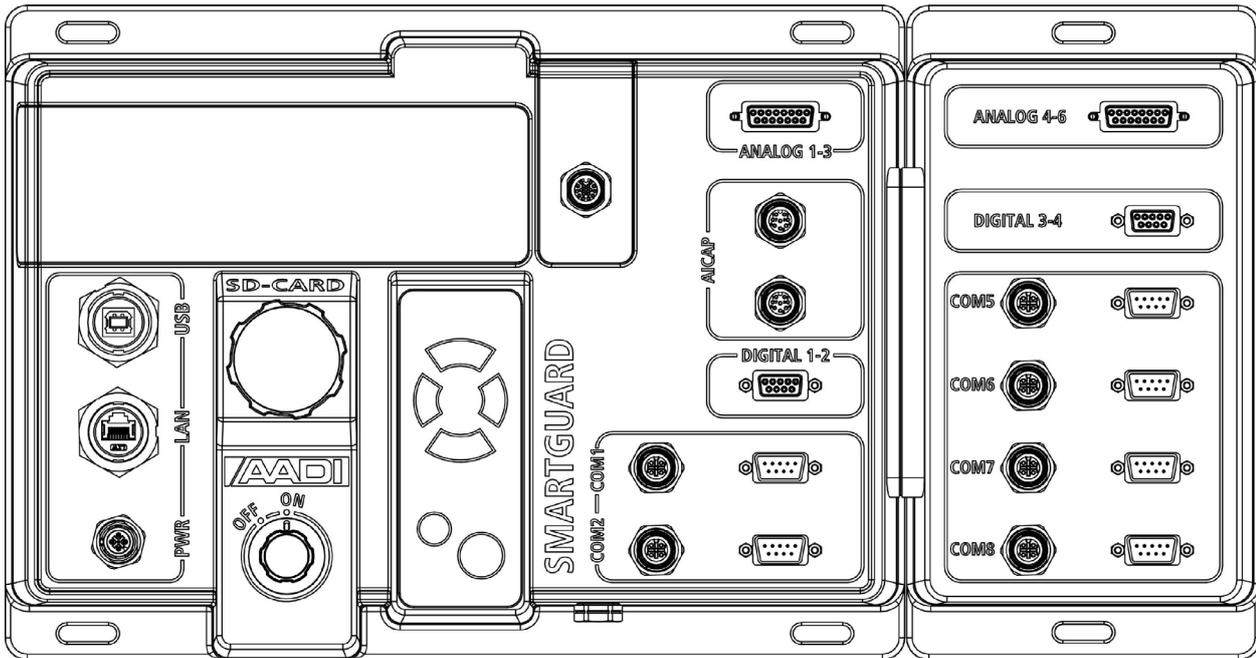
Figure A 1 The SmartGuard extended version connection plugs.
