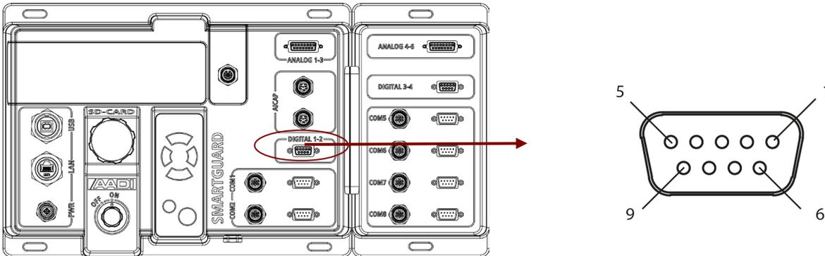
Figure A 5 9-pin D sub connection plug. Refer Table A 7 for signal wiring.
