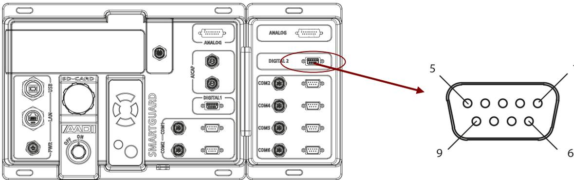
Figure A 12 9-pin D sub connection plug. Refer Table A 17 for signal wiring.
