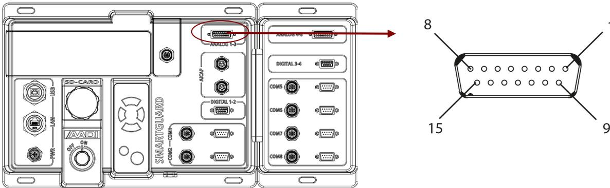
Figure A 6 9-pin D sub connection plug. Refer Table A 8 for signal wiring.
