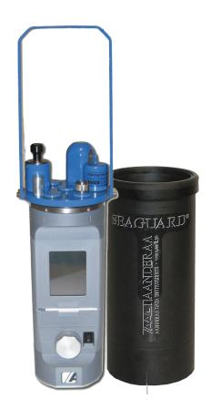
The SeaGuard CTD is a primary tool for determining essential physical properties of sea and fresh water. Standard parameters are Conductivity, Pressure/Instrument depth and Temperature. From these parameters the salinity of the water as well as the density are calculated.
