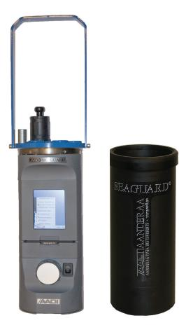
The SeaGuard Wave and Tide Recorder measures wave and tide conditions based on a silicon pressure sensor 5218. The pressure measurements are sampled and temperature compensated by an advanced Digital Signal Processor.
