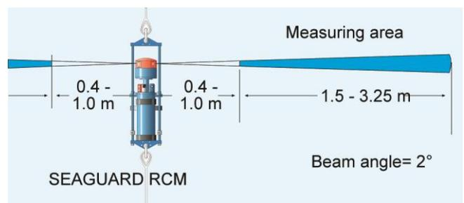
Figure 1-1 Measuring area of the SeaGuard RCM.
