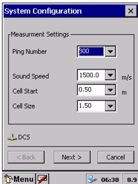
**Figure 2-1**Deployment Settings; set the Sound Speed, Cell Start and Cell size.
