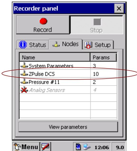
The ZPulse DCS provides 10 measurement parameters. These parameters are:
