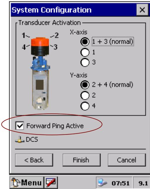
Figure 2-3 Transducer Activation.
