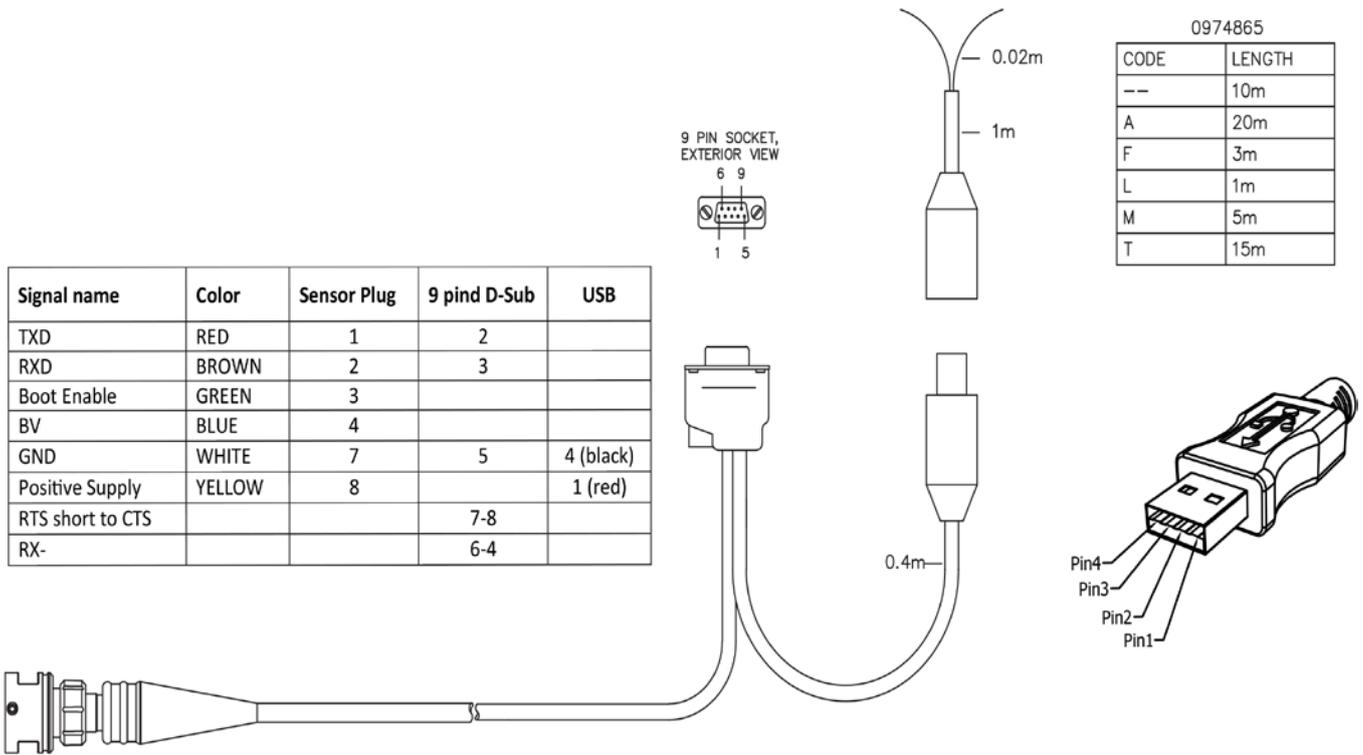
Figure A 7 Set up and configuration cable 4865, RS-232 for field use.
