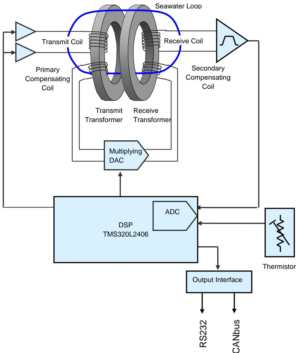
Figure A 5 Functional Diagram
