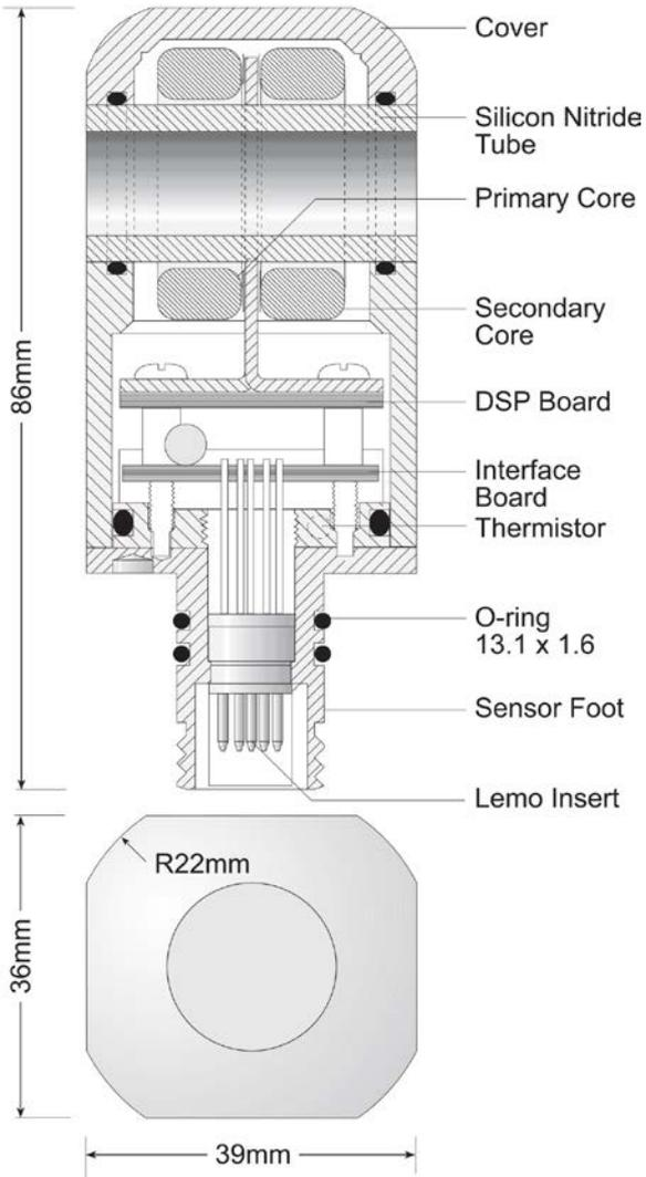
Figure A 2 Drawing of Conductivity Sensor 4319
