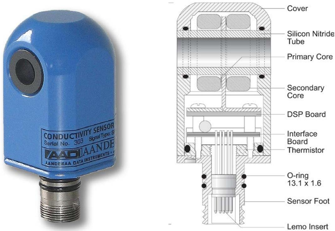
**Figure 1-1: Illustration of the Conductivity Sensor 4319**
