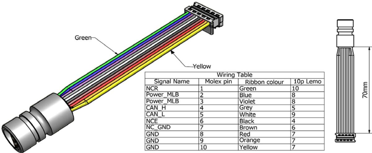
Figure A 11 Drawing Patch Cable 4999, AiCaP
