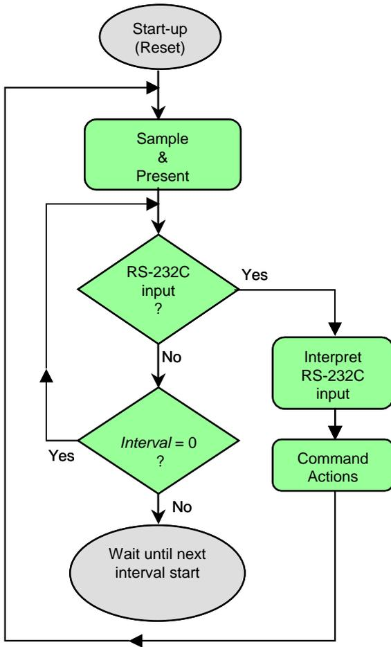
Figure 5-2 Software, RS232 operation sequence
