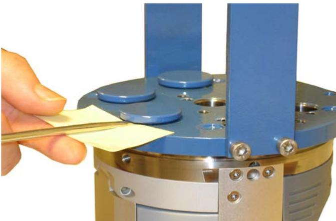
**Figure 3-2: Removal of sealing plug. Use a small piece of paper/cardboard to protect the lacquer of the top-end plate**
