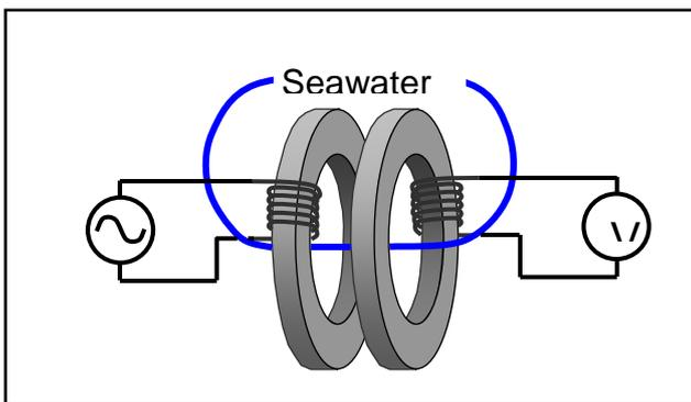
Figure A 4 Transmitter and Receiver Transformer
