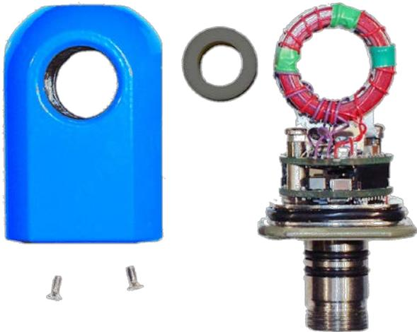
**Figure A 1** Conductivity Sensor 4319 Internal Components
