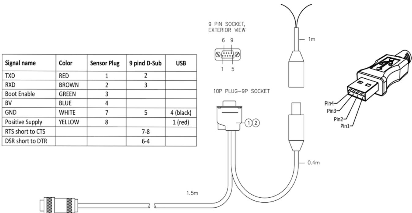
**Figure A 6 Set up and configuration cable 3855, for laboratory use.**
