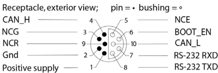
**Figure 1-2: Conductivity Sensor 4319 pin configuration.**
