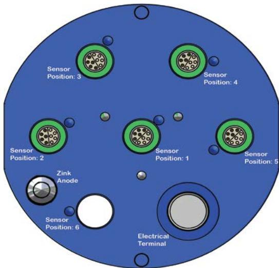
**Figure 3-1 Illustration of the SEAGUARD® Top-end plate.**
