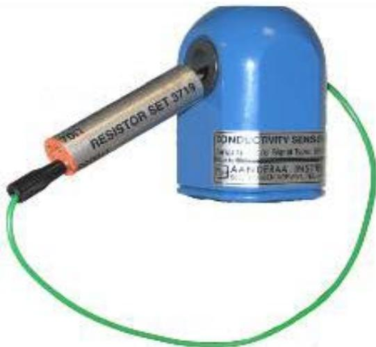
**Figure 6-1** Let the resistor wire go through the sensor hole and connect it in the 4 inlets on the other end of the resistor.
