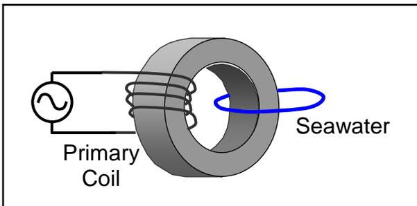
Figure A 3 Transmitter Transformer
