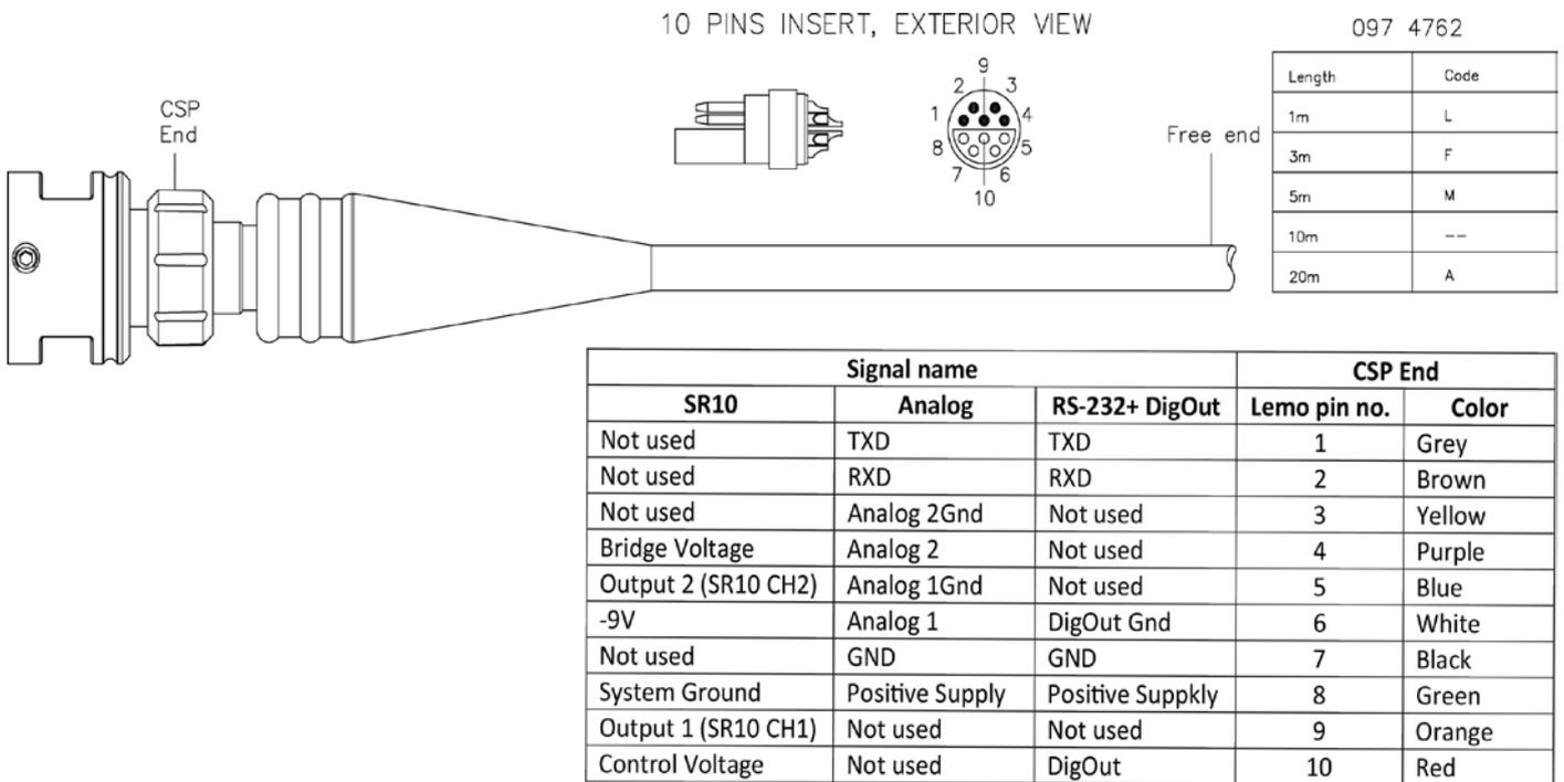
Figure A 8 Drawing Free end Cable 4762, RS-232
