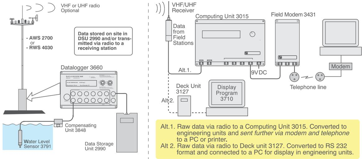
Illustration below shows a simple recording water level monitoring system which has a variety of applications. Water level monitoring in ports reservoirs, dams, ponds etc. are some of the areas which can be covered. Adding a VHF or UHF radio to the system will make a radio tide gauge.
