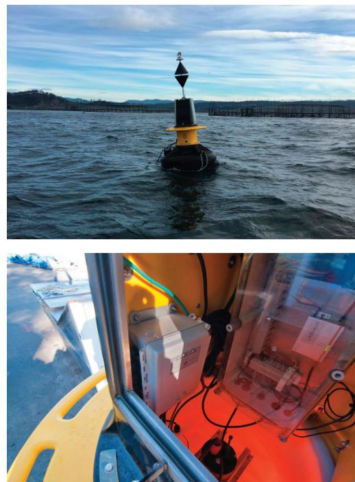
Instrumentation Bay in the top cavity of the Buoy, showing the MOTUS sensor below.
