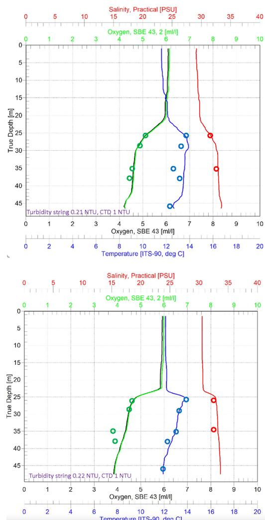
**Fig 4:** CTD-profiles close to the SeaGuardII mooring before deployment (left) and at the time of recovery (right). The Circles in the left profile indicate the oxygen (green), temperature (blue), and salinity (red) observations by the sensor string connected to the SeaGuardII instrument.
