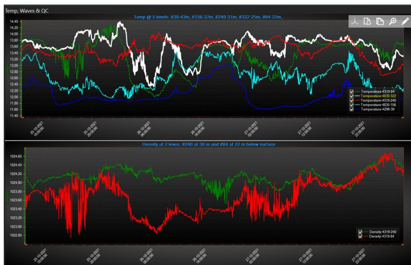
**Fig 3:** Continuous Temperature (upper graph) and Density (lower graph) measurements with string system. The green line in the density plot is from 35 m and the red from 26 m. Please note the variability and that at occasions, the density is similar at both levels, which indicates that the water is mixed.
