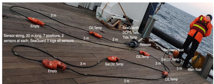
**Fig 1:** SeaGuardII string system laid out on deck before deployment. (Photo: Amanda Nylund)
