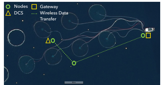
Overview of fish farm - sensor data relayed via underwater mesh network.
