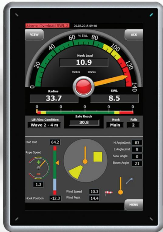
Sixth generation Safe Load Indicator, SLI/RCI/LML with comprehensive data logging and customized interface, flexible and configurable using touch screen technology
