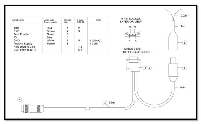
Figure 10-7: Set-up and configuration cable 3855
