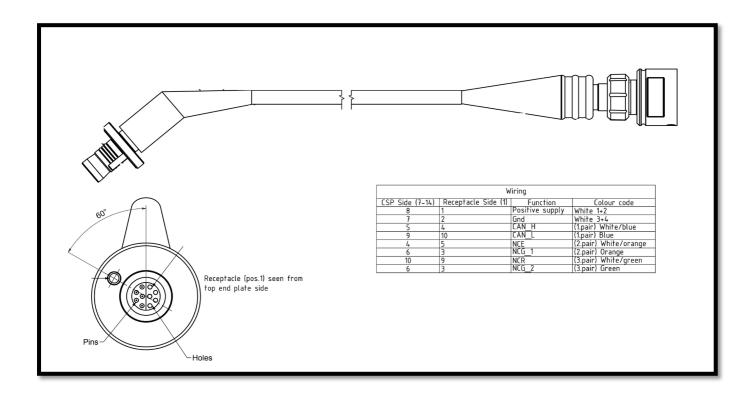
Figure 10-10: Remote sensor cable 4973
