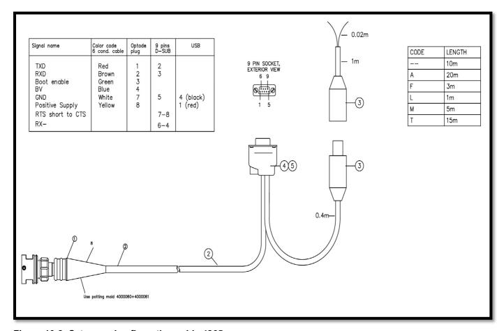
Figure 10-8: Set-up and cnfiguration cable 4865
