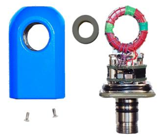
Figure 8-2: Sensor before final assembly
