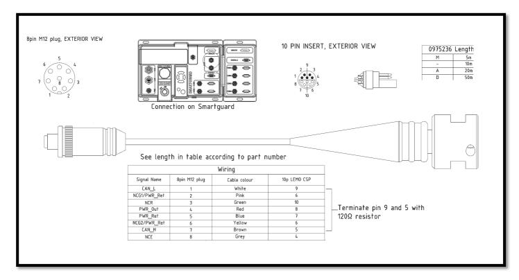
Figure 10-12: 5896 Sensor cable to SmartGuard
