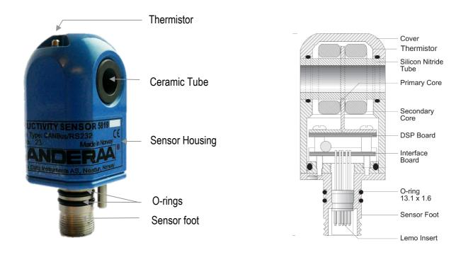
Figure 1-1 Illustration of the Conductivity Sensor 5819.
