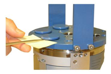
Figure 2-2: Removal of sealing plug.
