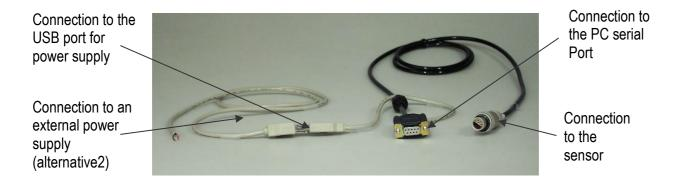
Figure 1-7: Set-up and configuration cable 3855
