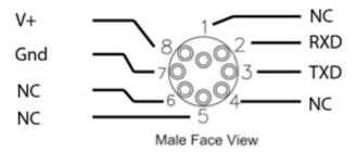
Figure 1-6: Pin Configuration Conductivity Sensor 5990
