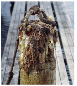
Figure 7-1: Example of fouling
