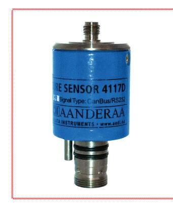
In most measuring systems used in the sea, pressure is a vital parameter. For moored instruments the pressure can be used for determining the actual depth of the instrument. For instrumentation on the seabed the pressure can be used for deriving water level. The pressure is also vital when deriving other parameters as density and speed of sound.
