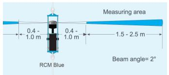
The solid state sensor is well suited for monitoring low current speeds due to no moving parts. Because the sensor starts measuring in an area 0.4 to 1.0 meter from the instrument, the effect of marine fouling and local turbulence is minimized.
