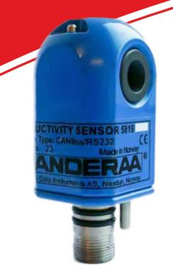
Conductivity Sensor 5819/5819R is a compact fully integrated sensor for measuring the electrical conductivity of seawater. Designed to be used with SeaGuard or SmartGuard data logger using AiCaP CANbus or as stand-alone sensor using RS-232/RS-422
