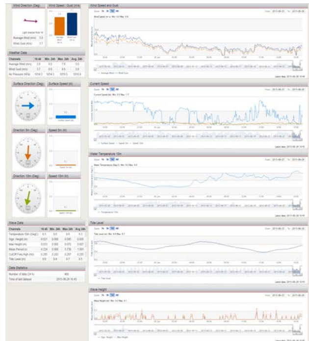
Fig. 15. Geoview real time data visualization web-based display
