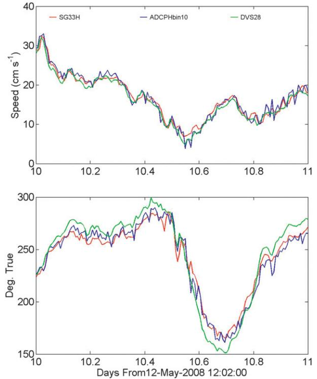
FIG. 5. Example of small but persistent DVS compass deviations: (top) speed and (bottom) direction.
