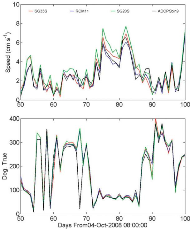
FIG. 7. Example of small but persistent SG20S overspeeding error: (top) speed and (bottom) direction.
