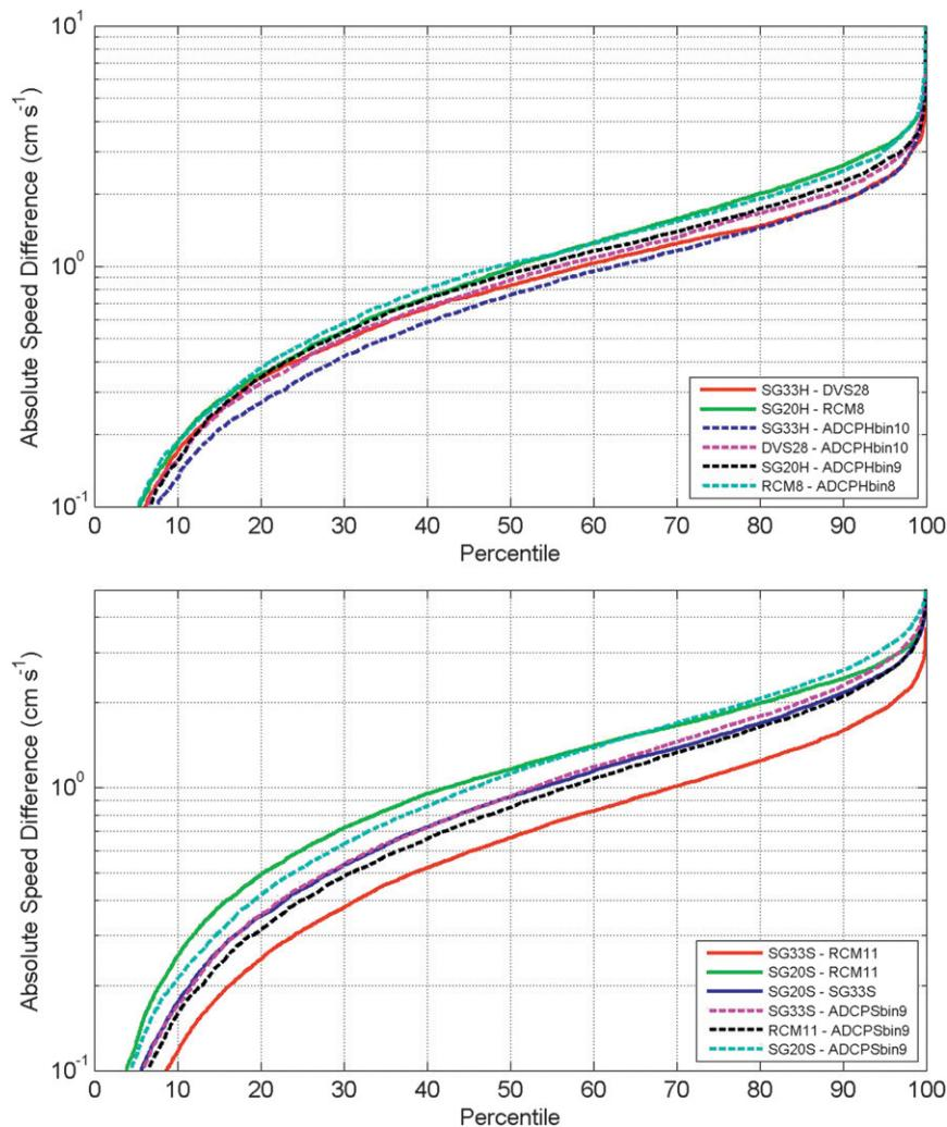
FIG. 9. Percentiles of instrument speed differences for (top) shelf and (bottom) slope deployment.
