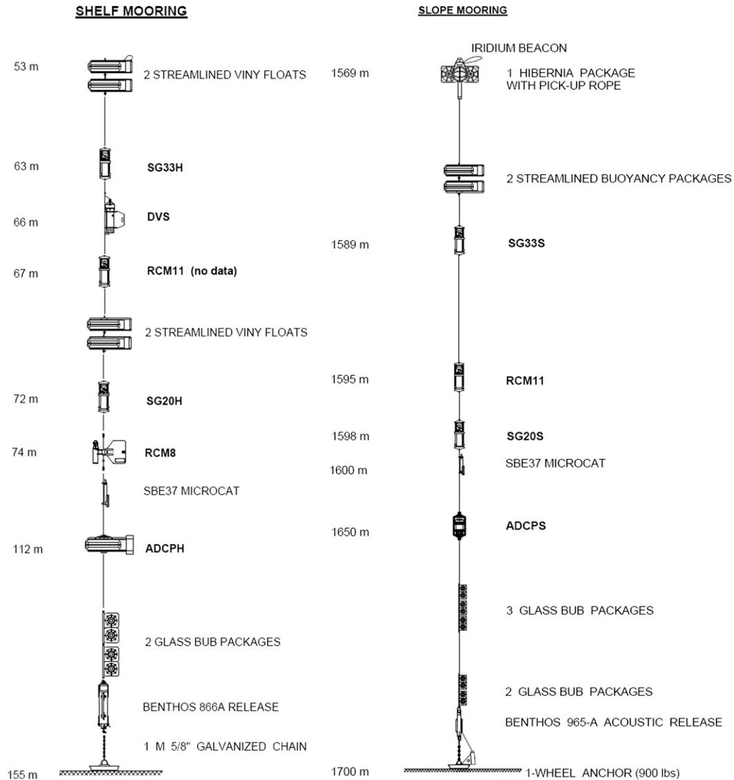
FIG. 2. Schematic of mooring layout used in the 2008–09 intercomparison experiment.
