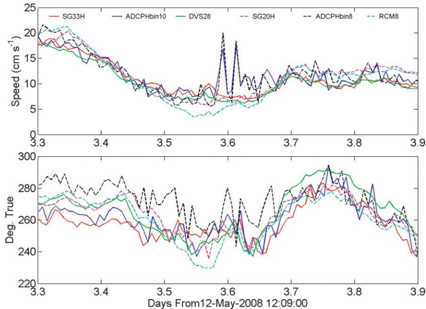
FIG. 13. Example of occasional large ADCP error in shelf deployment: (top) speed and (bottom) direction.
