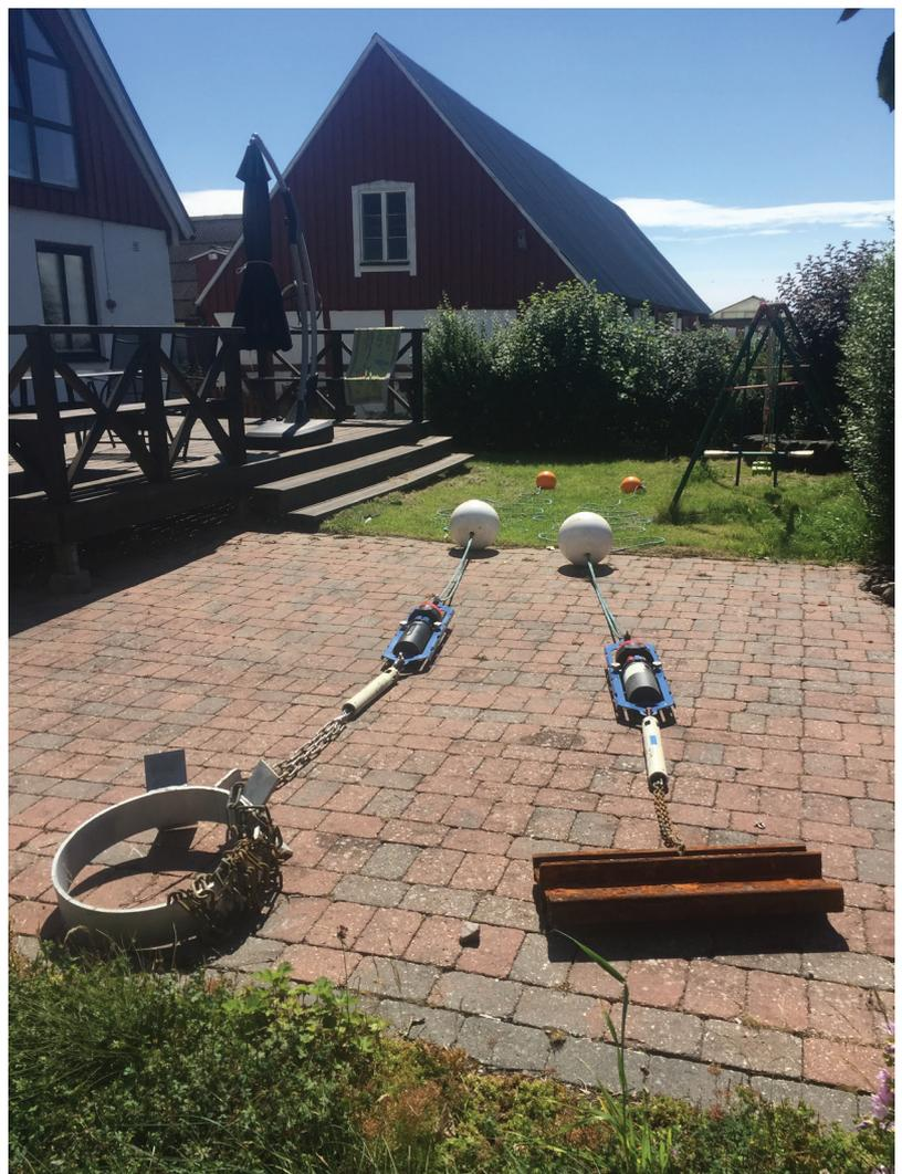
Fig1: Two instrument moorings prepared for deployment. Ballast weight at bottom, chain, acoustic release (thin grey cylinder), instrument, and two floats (white & orange) with lines.
