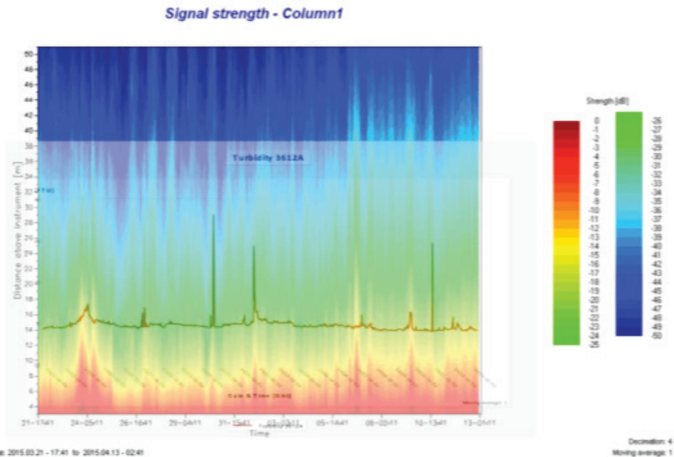
Fig 2: Overlay plot of [turbidity](#) measured about 1.5m above bottom (black line) and [acoustic backscatter](#) from the bottom up to 50m above (colour plot) from the Måseskär dumpsite. The occasional peaks in turbidity and backscatter correlate with each other and are all related to identified trawlers that fish in the area. No events of natural re-suspension due to high currents were detected.
