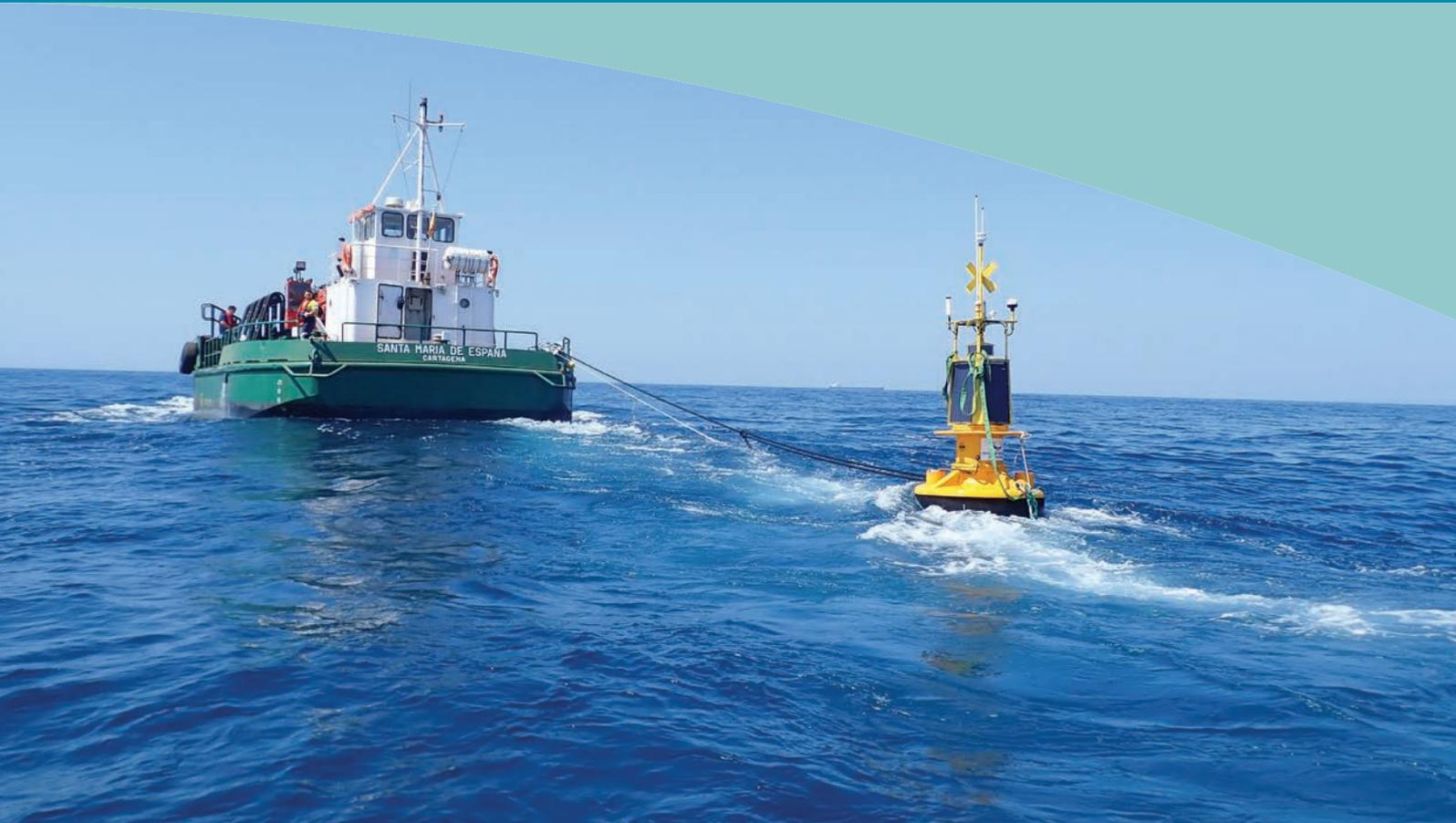
Fig. 1: Deployed SB-138 P buoy equipped with MOTUS wave sensor, DCPS, GMX200 weather sensor, and ATON AIS Type 3
