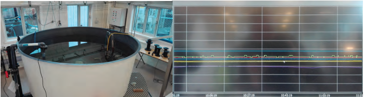
SOLVOX® Dropln and Twin Kit in test tank, as well as display of data logged during the oxygen measurement test
