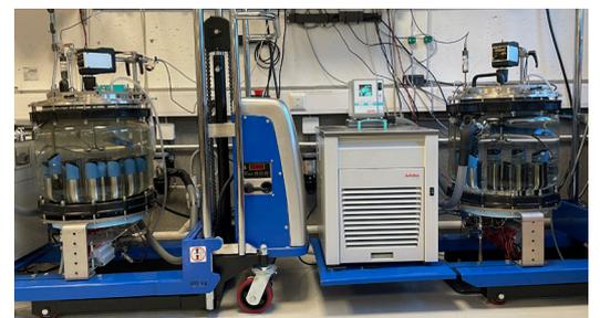
Figure 3: Oxygen multipoint calibration systems at Aanderaa
