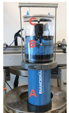
Figure 1: Pressure testing system. A. SeaGuard logger. B. Sensors in test water. C. Stirrer for incubator water mixing.
