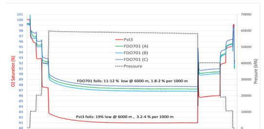
Figure 2: Short-term pressure effects on Pst3 and FDO701 foils.
