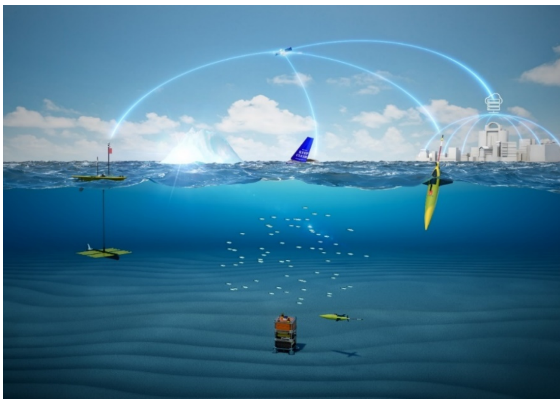
Unmanned ocean vehicles collect field data and transfer these via satellite to shore (3D visualization by Kongsberg Maritime).
