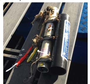
The acoustic recovery system of the mooring systems with the fishing lures
