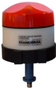
**Figure 2-1 The Doppler Current Profiler Sensor 5400.**
