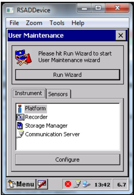
When you select **User Maintenance** you will first enter a window with a Run Wizard button on the top and then two tabs named **Instrument** and **Sensors**.
