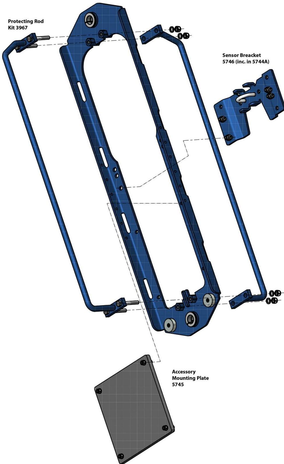
Figure 10-2: Inline mooring frame 5744A
