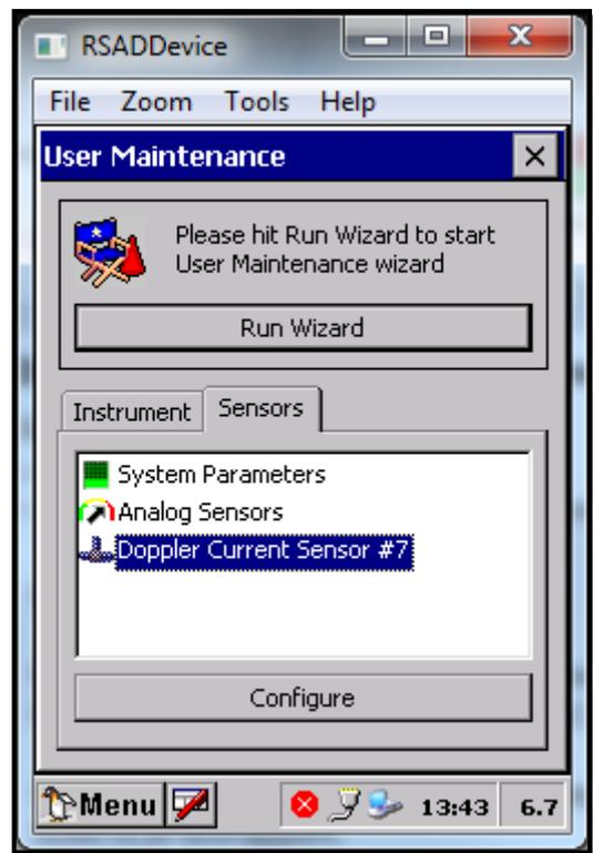
Select the **Sensor** tab and then the **DCS** before ticking the **Configure** button
