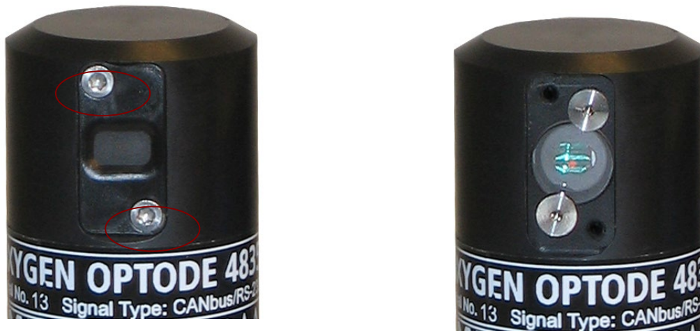
Figure 7-4 Removing the securing plate and change the sensing foil.
