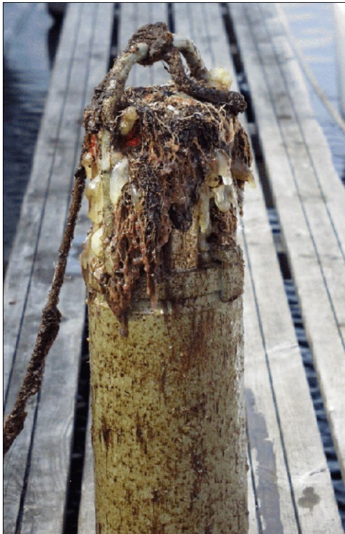
Figure 7-1: Example of fouling on an RCM 9 with an Oxygen Optode 3830 (Optode version with SR-10 output) mounted to it: The Optode was still giving correct readings.
