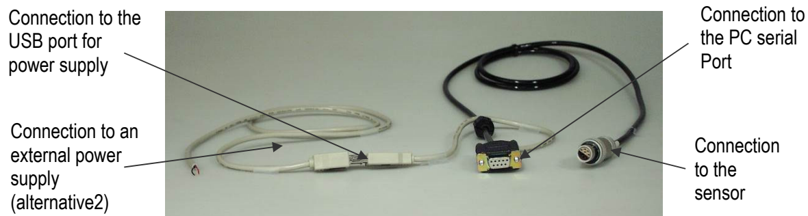
Figure 2-8: Set-up and configuration cable 5618
