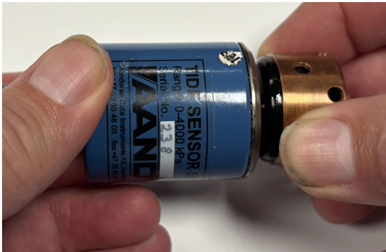
Figure 9-2: Mounting Pressure Inlet w/membrane to sensor
