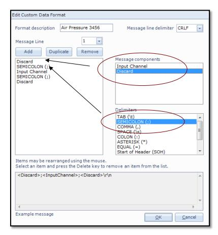
Figure 5-3 Specifying serial sensor data format.
