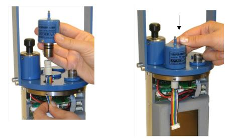
Figure 7-13 Connect the sensor to the patch cable 3969492.
