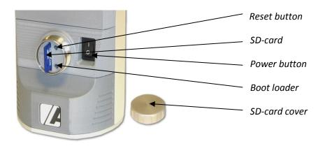
Figure 1-3 SD-card slot
