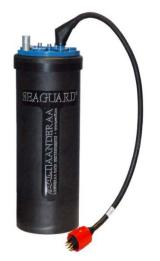
Figure 2-1 SeaGuardII with USB-configuration cable
