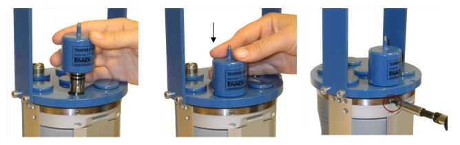
Figure7-11 AiCaP sensors: Place the sensor according to the orientation pin. Push down the sensor and fasten the set screw.
