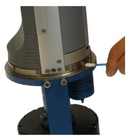
Figure 8-2 Clean O-ring seating; instrument up-side-down.
