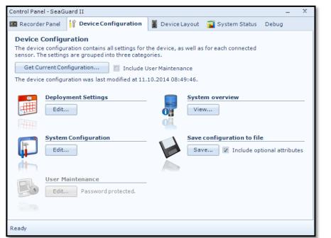
To start configuring the instrument, select the **Device Configuration** tab on the top row in the Control Panel, press "**Get Current Configuration...**" in order to get the actual configuration from the SeaGuardII.
