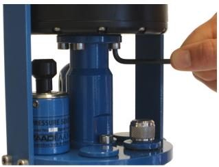
Figure7-15 Connect the ZPulse DCS / DCPS.
