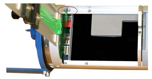
Figure 7-12 Open the battery lid, remove the upper battery, and unscrew the two top screws that holds the top front cover. Turn the instrument and pull off the top front cover.
