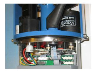
Figure 7-16 Connecting the 4784 Cable
