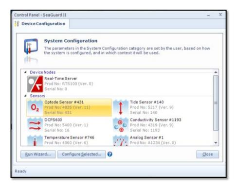
The system configuration can be changed using either a wizard ("*Run Wizard...*") which steps you through the settings of all available nodes or, by choosing a specific node to configure; click first on the node to modify and then "*Configure Selected...*"
