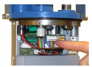
Figure 7-14 Connect the patch cable to HUB plug J6.
