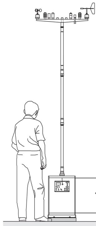
The average wind speed is obtained as the arithmetic mean of the wind regardless of the sampling interval, provided that the sampling interval is between four seconds and three hours.
