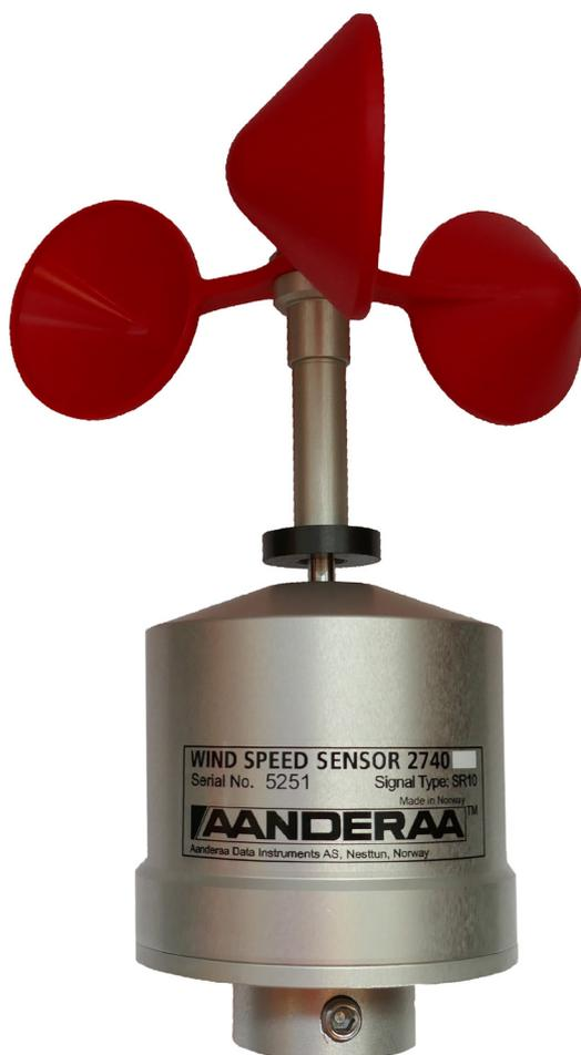
The Wind Speed Sensor 2740 consists of a three cup rotor on top of an aluminium housing. The sensor can be fitted directly onto the Sensor Cross Arms 3415/3435 of an Aanderaa automatic weather station or used separately if a connecting cable is used. The sensor foot will fit onto a 25 mm vertical tube.
